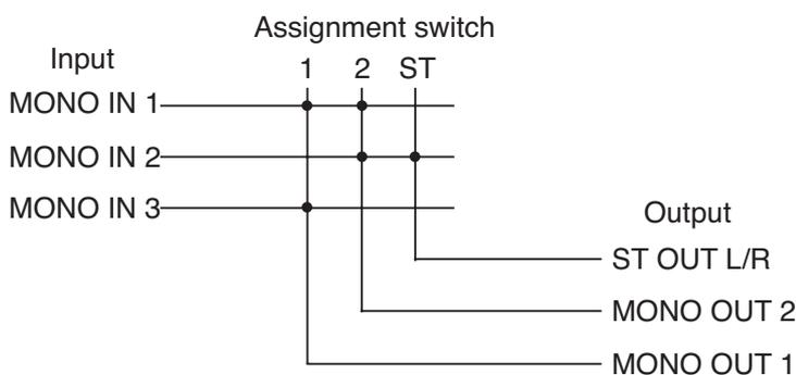
Mixed signals of the MONO IN 1 and MONO IN 3 are output from the MONO OUT 1, those of the MONO IN 1 and MONO IN 2 from the MONO OUT 2, and the MONO IN 2 signal from the ST OUT L/R.
