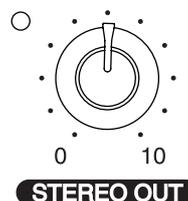
**2-3.** Adjust the volume level of the output amplifier connected to the STEREO OUT.
