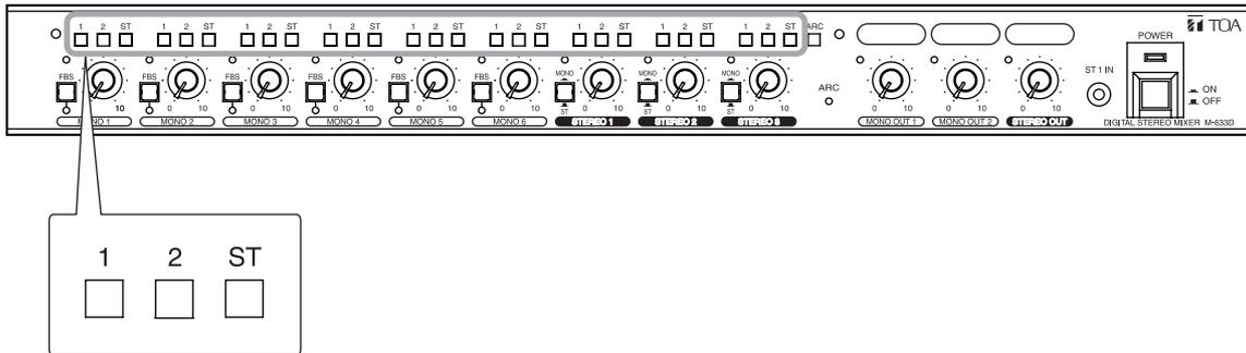
Pressing the Assignment switch "1" routes the input signal to the MONO OUT 1 output, switch "2" to the MONO OUT 2 output, and switch "ST" to the STEREO OUT output. Input signals assigned to the same output destination are mixed.
