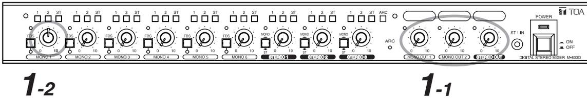
**1-1.** Turn all the output level control knobs to the "0" position.
