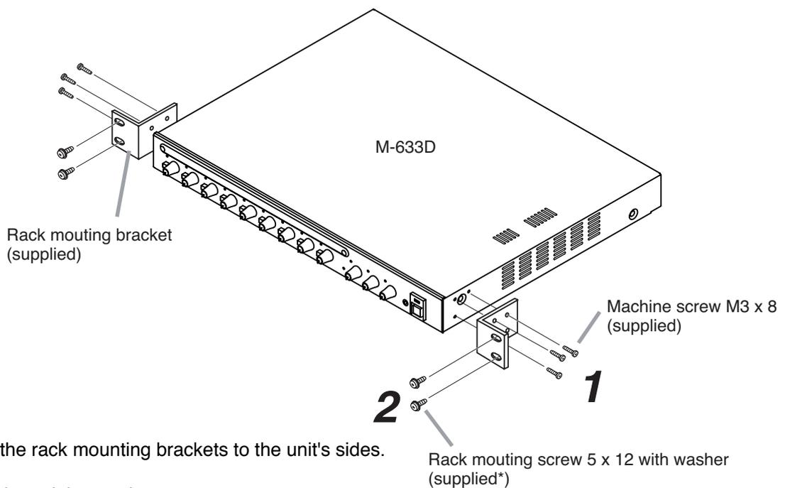
**Step1.** Attach the rack mounting brackets to the unit's sides.
