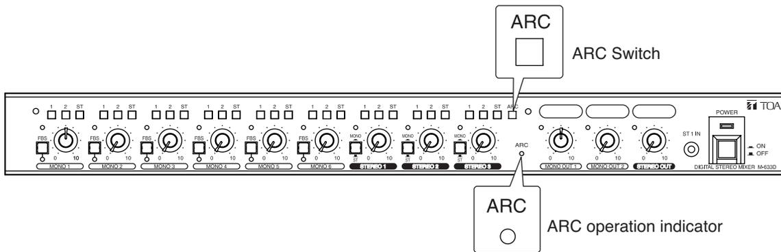
Hold down the ARC switch for 3 seconds.
