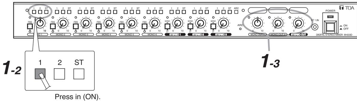
**1-1.** Turn the MONO 1's input level control knob to the 12 o'clock position.
