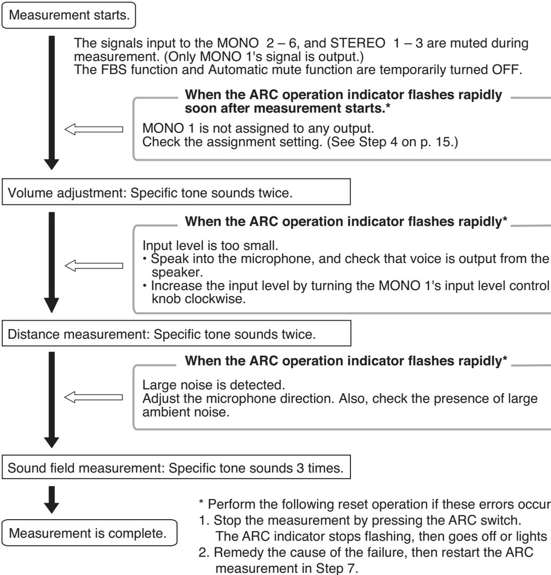
**Measurement is complete, and the ARC filter is set.**
