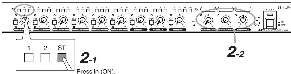
**2-1.** Press in only the MONO 1's assignment switch "ST" to turn it ON.
