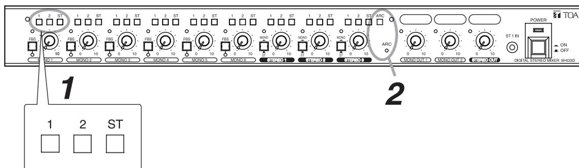
**Step 1.** Place the MONO 1's all 3 assignment switches in unpressed state.
