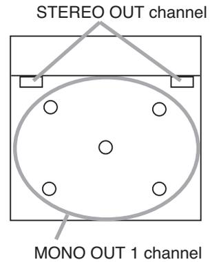
**Step 1.** Set the ARC filter only to the MONO OUT 1 channel (ceiling speakers).
